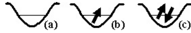
Figure 2. Electronic states in the inter-QPC island. We assume that there is only one accessible electronic orbital state on the island. There are thus in total four possible island states: (a) empty dot—state ‘a’ has no excess electron on the dot. (b) Single-electron dot—state ‘b’ has one electron with spin up or down. (c) Two-electron dot—state ‘c’ has two electrons in a spin singlet state occupying the same orbital state.
